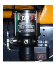
The system of centralized lubrication provides constant lubrication of components of the machinery, due to the system of progressive distribution. With this principle the desired quantity of lubricant can be distributed to each grease point, ensuring an excellent resistance to wear due to correct, measured and directed continuous lubrication of the machine.
